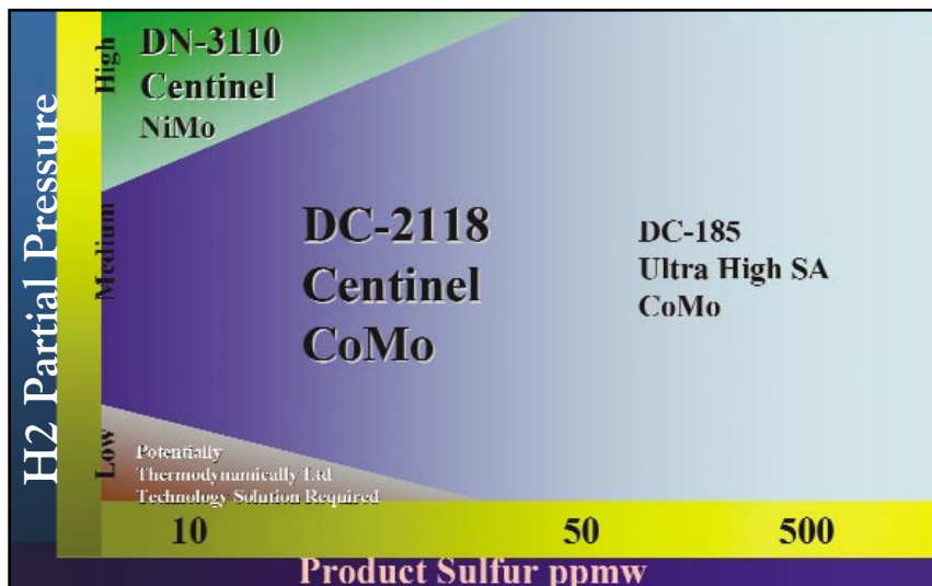
Figure 6. Application area for conventional vs. CENTINEL catalyst in distillate HDS.
